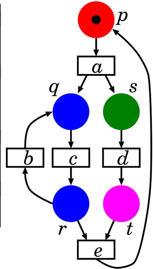
$$\mathcal{X}_4: \{p^0, p^1\} \equiv \{0, 1\} \quad \mathcal{X}_3: \{q^0 r^0, q^1 r^0, q^0 r^1\} \equiv \{0, 1, 2\} \quad \mathcal{X}_2: \{s^0, s^1\} \equiv \{0, 1\} \quad \mathcal{X}_1: \{t^0, t^1\} \equiv \{0, 1\}$$
