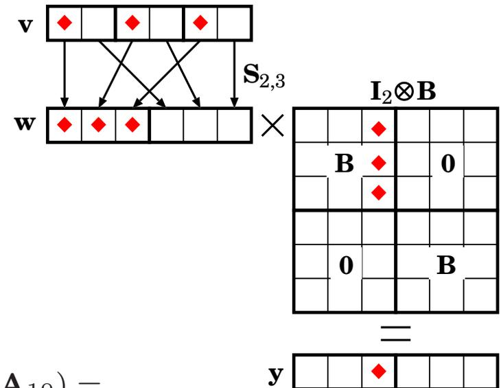
$$y \leftarrow \underbrace{x \cdot S_{2,3}^T}_{u} \cdot \underbrace{(I_3 \otimes A)}_v \cdot \underbrace{S_{2,3} \cdot S_{6,1}^T \cdot (I_2 \otimes B)}_w \cdot S_{6,1} = y$$
